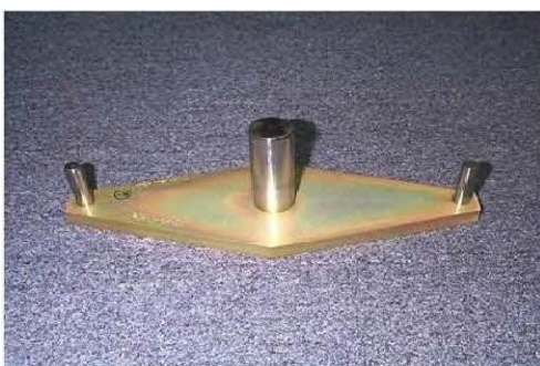
212/412 Tail Rotor Hub Trunnion Centering Tool HTI011
