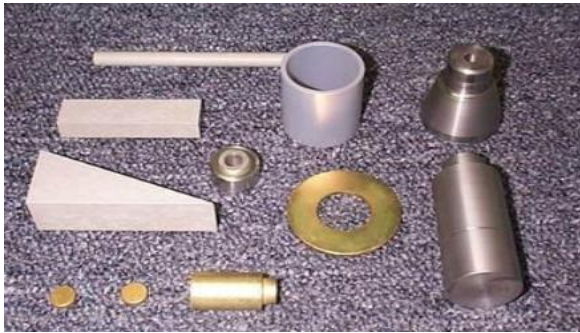
Main Rotor Trunnion Inner Race Removal Work Aid HTI020
