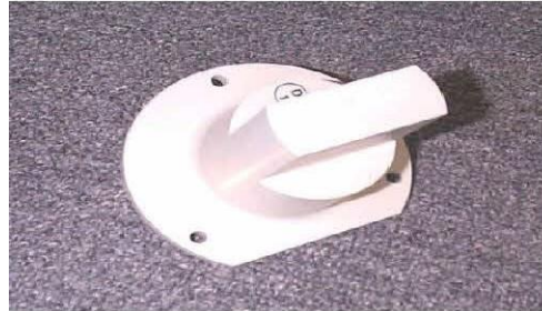
412 HP/EP Tail Rotor Output Adapter Backlash WA HTI013
