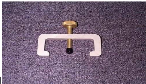
212/412 Tail Rotor Hub Trunnion Centering Tool HTI011
