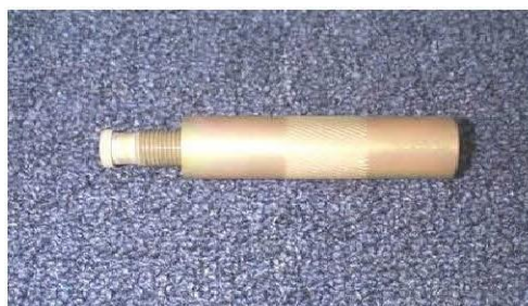
204/205/212/412 Swashplate Gimbal Ring Bolt Removal Tool HTI012
